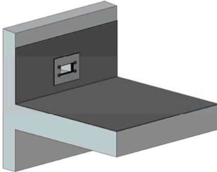
Set the spring rings and hex nuts on the threaded pins and tighten the nuts diagonally (max. torque 8 Nm).
