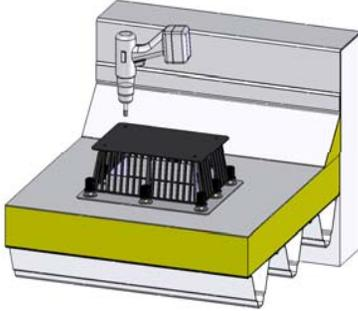
Lay the cover plate on the dome grate and align them that the holes of the cover plate are laying directly above the holes of the dome grate. Mount the cover plate with the enclosed screws.
