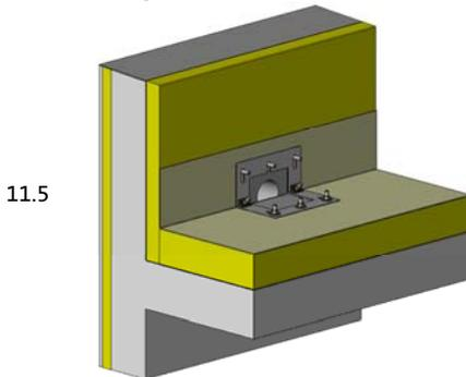
Push the washers  $\varnothing$ 36 mm over the threaded pins on the loose flange in the sealing layer. Apply the nuts and tighten alternating with a torque of max. 30 Nm.
