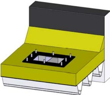
Set up the large rubber sealing sleeve over the threaded pins on the thrust-flange of the SitaTurbo.
