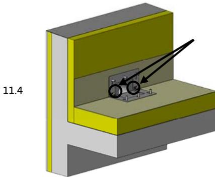
Push the bulkheads and the washer  $\varnothing$  24 mm in the edge areas of the SitaRondo over the threaded pins on the loose flange. Apply the nuts and tighten alternating with a torque of max. 30 Nm.
