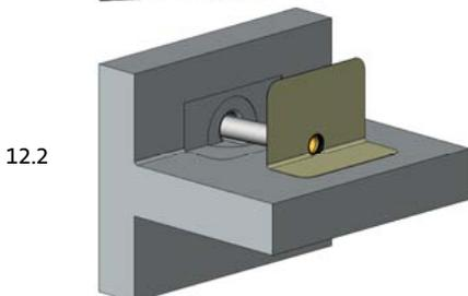
Push the SitaEasy with connected connection pipe through the core drill into the parapet.
