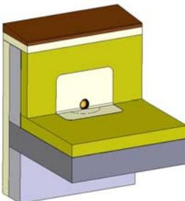
Grease the lamellar of the steam vapour barrier flex as well as the pipe of the component with lubricate. Push the pipe through the lamellar of the steam vapour barrier flex and insert the component to the determined position into the flat roof construction. The component needs to be fixed mechanically.
