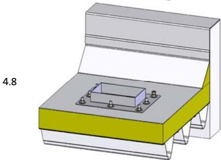
Lay the washers over the threaded pins on the loose-flange. Put the nuts on and tighten them diagonally and alternately with a torque of max. 30 Nm. According to DIN 18195 is a loose-thrust-flange construction at least three times to be controlled and tighten up in a timing of > 24 hours.
