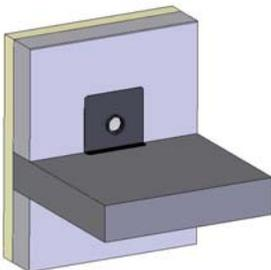
Mount the SitaSteam vapour barrier flex centrally on the facade breakthrough.
