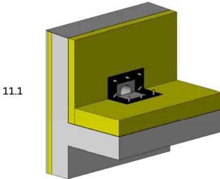
Put the Sita rubber sealing sleeve large over the threaded pins onto the thrust flange of the SitaRondo. In case of a bituminous roof sealing a rubber sealing sleeve is not necessary. Grease the thrust flange with bitumen primer and weld the bitumen track (tracks) on the roof structure.
