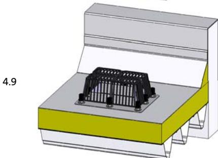
Lay the dome grate over the threaded pins on the nuts. Lay washers and nuts up and tighten them tangibly. Press the caps on the nuts.
