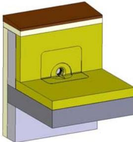
Cut out the contour of to be incorporated component from the thermal insulation and apply it to the roof area as well as the parapet.
