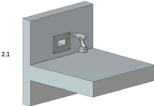
Secure the thrust-flange of the SitaTurbo Steam vapour barrier plate rigidly in front of the provided recess on the attic.
