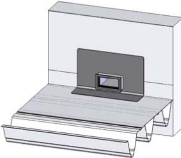
Mount the SitaTurbo Steam vapour barrier flex in front of the parapet recess.
