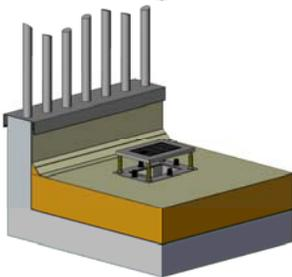
On terrace floorings above 93 mm the terrace installation kit adapter for extension have to be screwed in between the frame of the terrace installation kit and the brass bushings.
