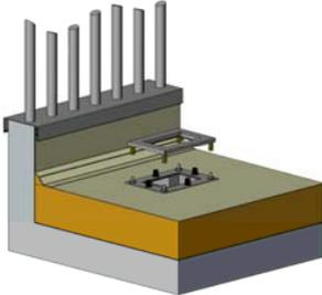
Place the SitaTurbo terrace installation kit with the four brass bushings on the four remaining threaded pins and adjust them to the desired height.
