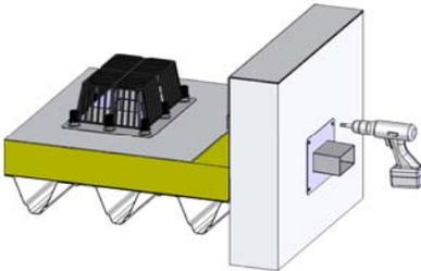
Place the cladding-cover plate over the out of the facade standing rectangular pipe of the SitaTurbo and fix it mechanically.
