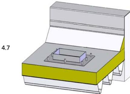
Heat the roof track and lay the loose-flange over the threaded pins on the small sealing sleeve.
