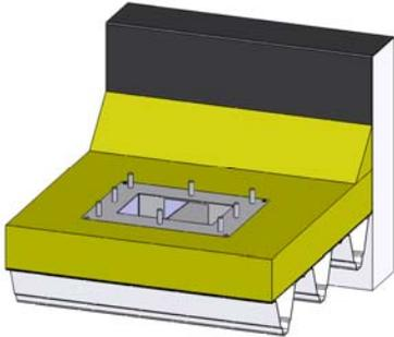
Apply to the rectangular pipe a wedge-shaped part of the cutted thermal insulation and adjust so that a flat surface is formed.
