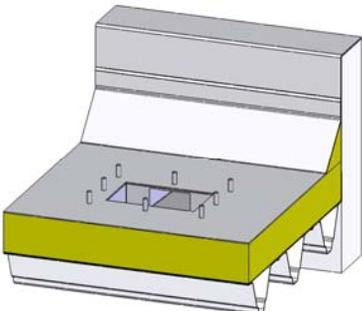
Determine the position of the SitaTurbo in the roof track. Use The loose-flange as template for the hole pattern of the threaded pins of the SitaTurbo.
