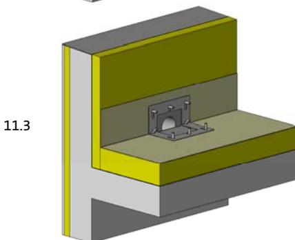
Lay the Sita rubber sealing sleeve small over the threaded pins on the roof track. Heat the roof track and lay the loose flange over the threaded pins on the Sita rubber sealing sleeve small.
