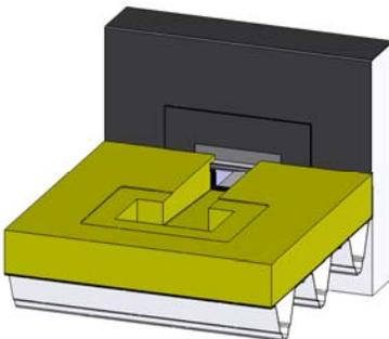
Cut out the contour of the SitaTurbo Attika outlet from the insulation. Place the thermal insulation onto the vapour barrier.
