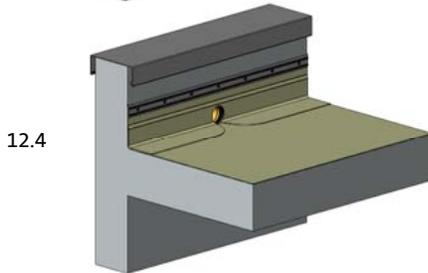
Glue or weld the roof track (tracks) onto the SitaEasy connection sleeve.
