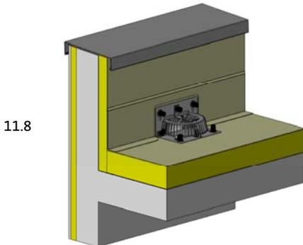
According to DIN 18195 is a loose-thrust-flange construction at least three times to be controlled and tighten up in a timing of > 24 hours.
