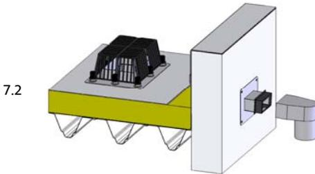
Grease the lamellar sealing from the outside and the stainless steel transition piece from the inside with lubricant.
