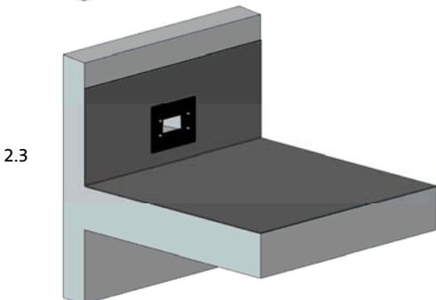
Postpone the connection sleeve over the threaded pins up to the vapour barrier.
