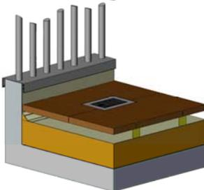
Insert the grid into the terrace installation kit frame. The terrace flooring can be fitted to the terrace installation kit.
