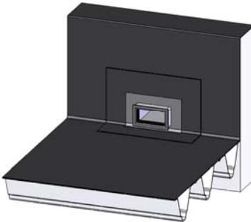
Define the position of the steam vapour barrier plate in the vapour barrier and cut out in such way that the vapour barrier can be connected vapour-tight to the vapour barrier plate adhesive flange.
