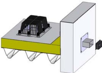
Place the lamellar sealing of the SitaTurbo outlet transition piece on the pipe end of the rectangular pipe and postpone it so much, that the stainless steel pipe lays in the three-sided U-profile. It is important to ensure that the pipe without U-profile is directed downwards.
