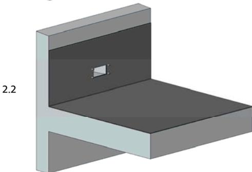
Define the position of the steam vapour barrier plate in the the vapour barrier. Punch out the hole pattern with a punch and postpone the vapour barrier over the steam vapour barrier plate up to the thrust-flange. Cut out the vapour barrier inside of the thrust-flange.
