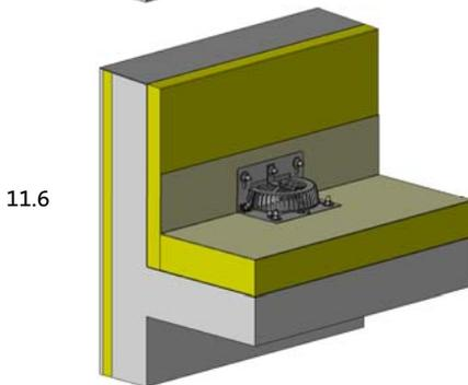
Put the dome grate with the angle bracket on the middle threaded pin in the parapet layer. Push the washer  $\varnothing$ 36 mm over the threaded pins on the loose flange or respectively angle bracket. Apply the nuts and tighten alternating with a torque of max. 30 Nm.
