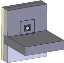
Glue the vapour barrier on the adhesive flange of the flexible steam vapour barrier.
