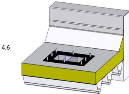
Lay the small rubber sealing sleeve over the threaded pins on the roof track.
