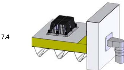
Postpone the on the facade mounted coupler downpipe on the transition piece.
