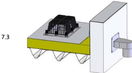
Postpone the transition piece over the lamellar sealing so much that the protruding lamellar lays from all sites in the transition piece. (See following detail).
