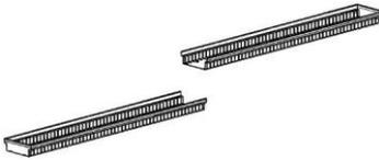
Place the drainage channel of the SitaDrain® Box drain, with inserted SitaDrain® Box drain head ends, on the roof construction.
